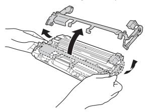
Using both hands, hold each drum and toner cartridge assembly level, and gently shake it from side to side several times to distribute the toner evenly inside the assembly.
